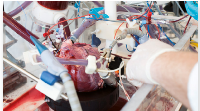
"LVAD connected to the apex of the PhysioHeart to study circulatory support strategies"
